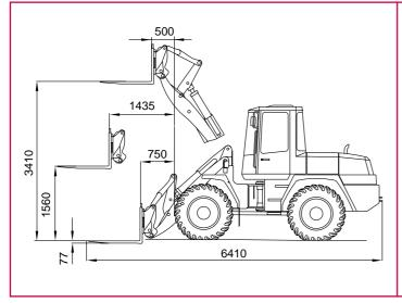
Payload over the total lift and steering range: 3000 (3250\*) kg Payload in transport position: 3250 (3500\*) kg
