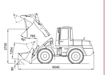
Capacity acc. to ISO 7546: 1.20 m<sup>3</sup> Density of material: 1.6 t/m<sup>3</sup>
